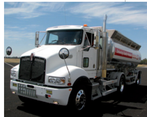
FUP prevents cars being trapped underneath.
